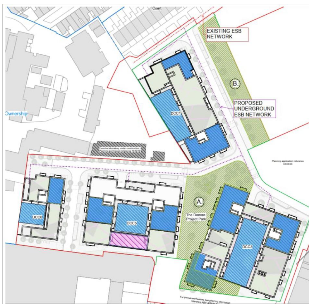
Figure 12-25: Existing & Proposed ESB Network (Source: AECOM, 2022, Mechanical & Electrical Planning Application Report)
